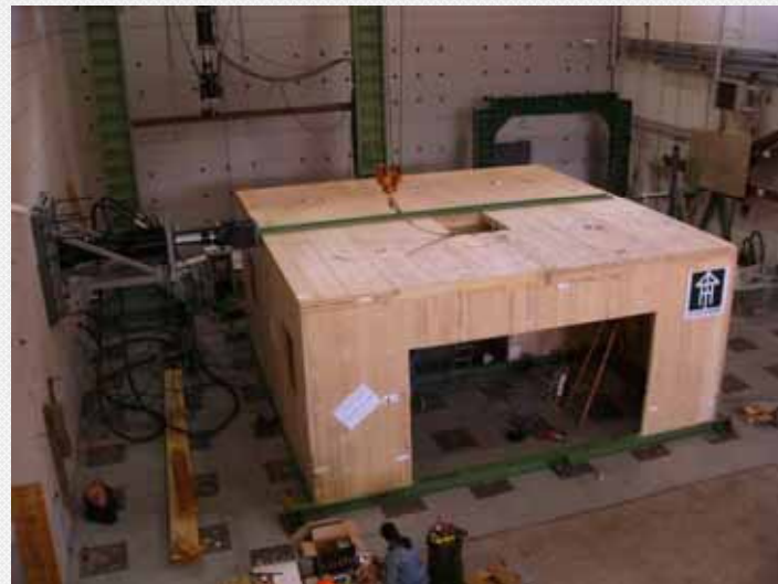
Pseudo- dynamic tests on one storey specimen
