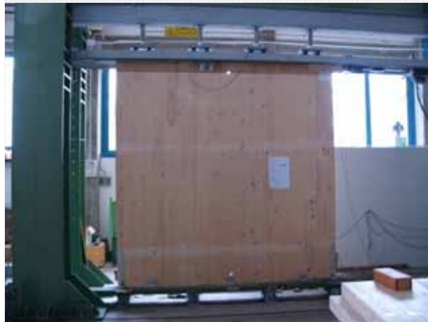
In plane Cyclic Tests on walls and connections
